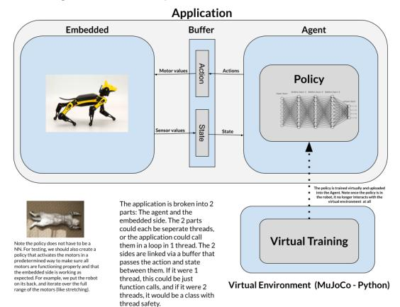
In addition to the text in the image, another important note is that this mimics a typical control theory system. The embedded side acts as an environment that has a state and accepts an action. The agent can contain any policy that makes decisions based on the current state. In addition to the above design, we have some basic pseudocode that will be implemented:
